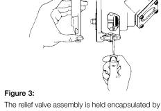
The relief valve assembly is held encapsulated by the screwdriver. You should now have both hands free to bolt down the cover. Insert and snug two bolts 180° apart to hold the cover. Finish inserting the remaining bolts and snug up evenly alternating until secure. Remove the screwdriver.
